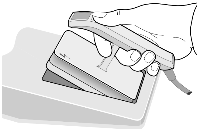
Figure 4-8. Returning the paddles to their compartments
